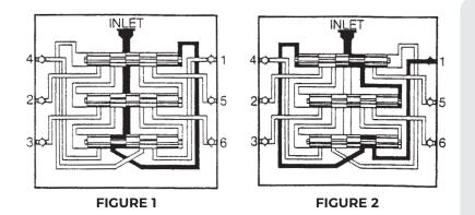
FIGURE 3 FIGURE 3 FIGURE 4 **FIGURE 1:** The inlet is connected to all piston chambers with only one piston free to move at any one time. With all pistons at the far right, lubricant flows against the right end of piston 1.
